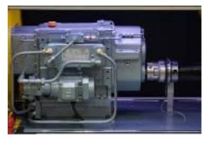
The water-cooled motors are of a new type from Austria which ensures a very efficient cooling and also minimize the size. An additional advantage with this motor type is that it has no fan and thus is not blowing air on to the body of the twin causing dust contaminations when running very dusty compounds.
