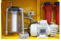
The 32 L/D extruder is, as standard, supplied with a vacuum zone on one of the barrel modules and the 40 and longer L/D versions also have an additional atmospheric vent opening which can be converted to vacuum. The vacuum vent zone has a stainless steel vent
