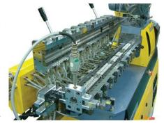
compound to another. The water cooling is done from fine channels inside each barrel module and regulated with individual solenoid valves from its designated temperature controller.
