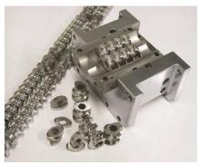
The screws are built on hexagonal elements is supplied in screw The modular Clam-shell Barrel is supplied as standard in the high temperature versions and it is equipped with exchangeable barrel lining inserts for optimum economy and ease of replacement. These standard inserts are made from a high grade tool steel which is through hardened to over 60 RC as well as nitrided for a surface hardness of 65 to 70 RC. The barrel with inserts can withstand high processing temperatures of up to 400 °C.
