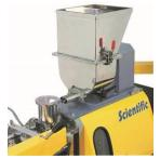
the side of the barrel module. A special barrel module with opening as well as plug for side feeder is needed for this option, and the extruder can be supplied with several plugged side feeder modules for optimum flexibility of side feeder location. The side feeder has an infinitely variable speed drive with 20 mm diameter twin screws and with an L/D ratio of 10. The entire barrel of the side feeder is equipped with water cooling as standard.
