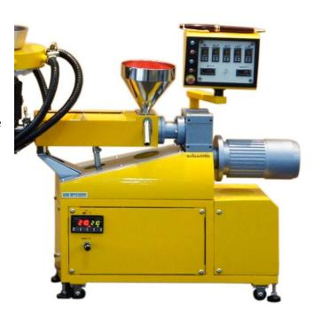
The hopper has a turret valve, same as with our larger extruders and it has a discharge pipe on the side to empty out the hopper.
