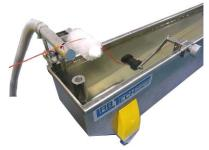
**Water bath** bench top type made of stainless steel with two strand rolls equipped with quick locks mounted on one side of the water bath so that the rolls can be placed in numerous positions for optimum cooling efficiency. The water bath is equipped with strand suction for efficient removal of all water on the stands. The vacuum device is built into the lower sub cabinet.
