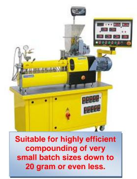
This twin is designed to be used with polymers in powder or micro pellets form with an approximate maximum granule diameter of 1.5 mm. It is suitable for processing of minute polymer quantities for research applications but it can also produce larger quantities having a maximum output of around 4 kg/hr. The amount of resin remaining in the screws is only around 10 grams so if the batch size is for instance 50 gram, the amount of polymer which is compounded and exits through the die is 40 gram.
