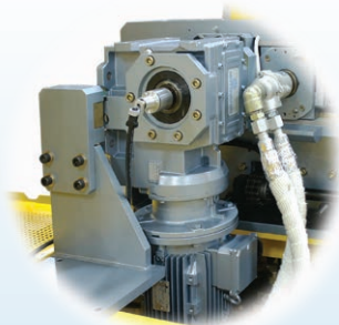
HEAVY DUTY DIRECT DRIVES TO THE ROLLS
