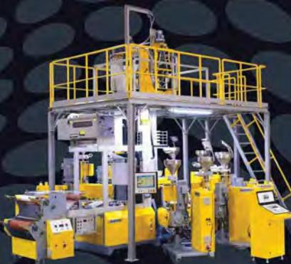
9-layers blown film line using two 30 mm and seven 25 mm extruder 30 L/D with Gravimetric hopper feeders and Dual channel high efficiency air ring, Stabilizing film bubble cage, Film bubble size controller, Oscillating nip roll.
