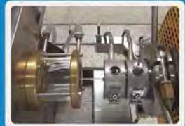
A 4-meter long filament calibration water bath is comprised of a stainless steel vacuum sizing/cooling tank and calibration bath equipped with water heater. The Vacuum section with heavy duty hinged Plexiglas lid and quick vacuum release valve mounted on top of the lid. It has a calibration tube inside the vacuum chamber and a venturi strand suction units at the end of the water cooling bath.
