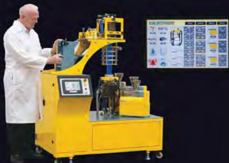
**The Ultra Micro 3-Layers Co-Ex Blown Film Line with 3 extruders**
