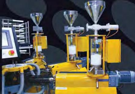
Our equally amazing 8 mm ultra micro extruder that can be fed with regular pellets with L/D Ratio of 30 and option of 40 L/D
