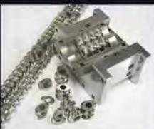
Single elements mounted on hexagonal shafts of screws for optimum flexibility of screw configurations.
