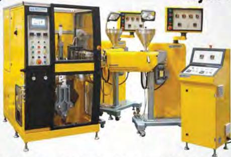
The Larger Bottle Blow Moulding attachment can be equipped with a 250 ml bottle mould of your own design
