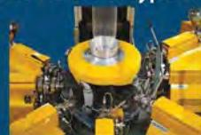
Oscillating Nip-Roll Haul Off with A-frame
