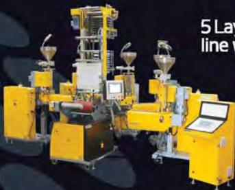
5 Layers Co-Ex film blowing line with 5 extruders
