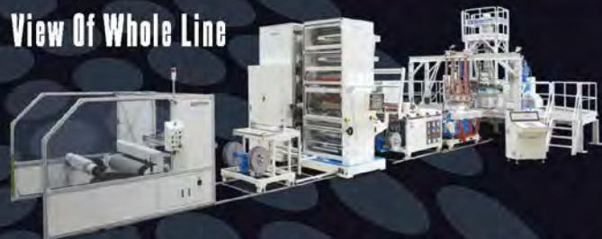
The line will be used for a multitude of polymers from polyolefin to more advanced thermoplastics like PET etc. It is equipped with two single screw extruders and one twin, feed block, die and a new design of a chill roll attachment with large 600 mm diameter rolls. Downstream the line has a new large vertical MDO unit as well as a wind up unit with automatic change over of the film rolls.
