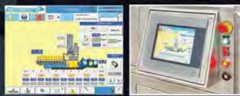
The main screen shows all the extruder functions. Controls can be made in compliance with 21 CFR Part 11 regulations.
