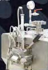
The Clam Shell Barrel is equipped with exchangeable barrel wear lining inserts for optimum economy and ease of replacement. These standard inserts are built to GMP standards in stainless steel with a focus on a clean.
