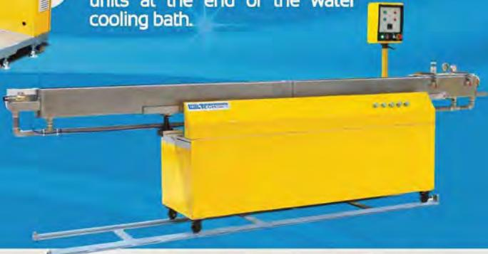
**4.0 meter length stainless steel vacuum sizing/cooling and calibration bath with water heater**
