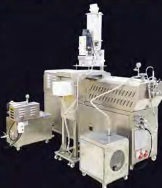
Closed Loop water circulating unit with heat exchanger and Vacuum pump system.
