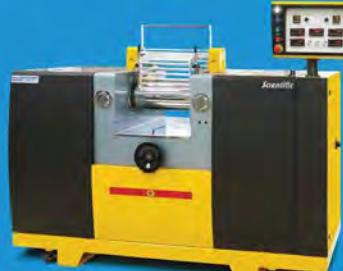
Rubber mills with water cooled or oil heated and cooled rolls. With variable speed heavy-duty direct drives to the rolls.
