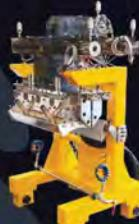
The Feed Blocks supplied with our co-extrusion lines are made for up to 9 layers
